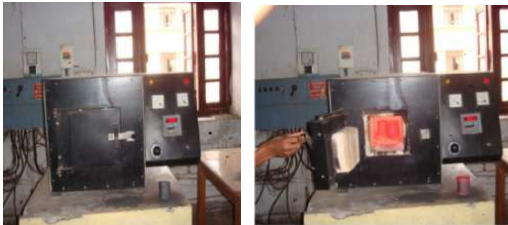
Fig 1: Carburization of Mild steel specimen in muffle furnace
